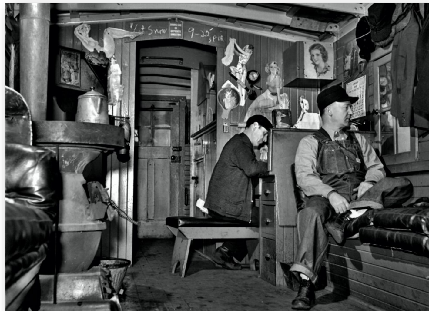
Photographed is the interior of a wooden caboose in January of 1943, according to close examination of the calendar on the wall. Another wall displays decorative images of attractive females, some in various stages of undress. The conductor works at his desk, while a brakeman, wearing his ubiquitous bib-front overalls, sits on a bunk nearby. Also, note the coffee pot on the pot-belly stove, the galvanized container beside it holding coal for its fuel, the coal stains on the floor, another bunk bed beside the stove, and the edge of the seat up in the cupola close to the top of the photo. A caboose was not always as clean, neat, or entertaining as this one, which created its common nickname as the "crummy." Garland Landmark Society Archives
